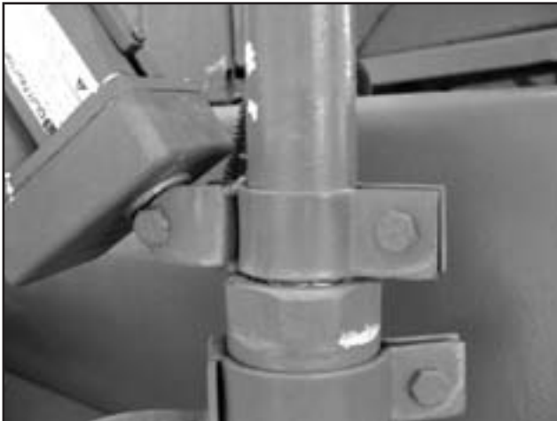
Actuator clamps to be fabricated from 1/8" x 1" flat stock
