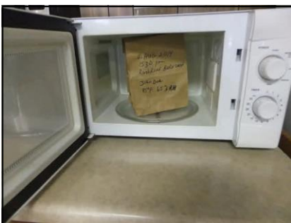
Figure 3. Sample drying in a microwave oven.
