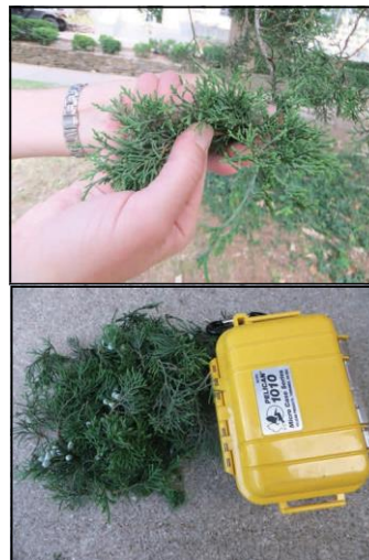
Figure 1. Collect cedar leaves by hand, avoiding any woody stems or branches when measuring fuel moisture.
