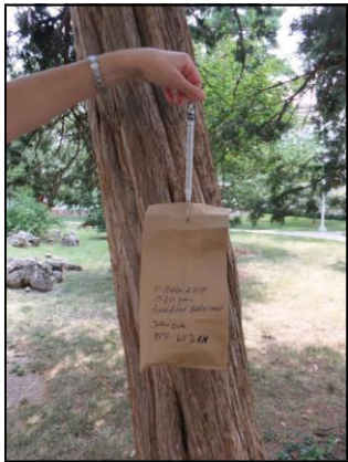
Figure 2. Sample bag with label being weighed with a spring scale in the field.
